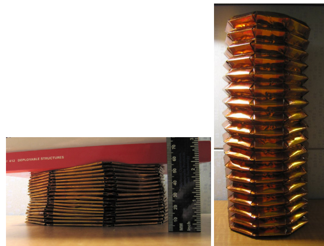
Figure 10 – Scale model of accordion-style shroud
